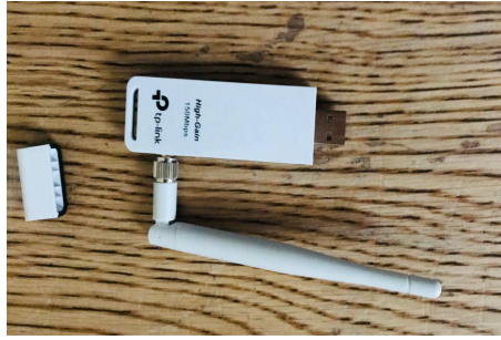
Figure 55. TP-Link (TL-WN722N) USB Adapter
