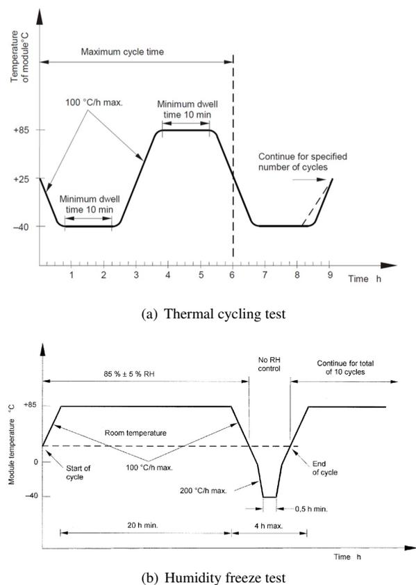
**Figure 1.** Accelerated ageing tests prescribed by IEC standards<sup>20</sup>.
