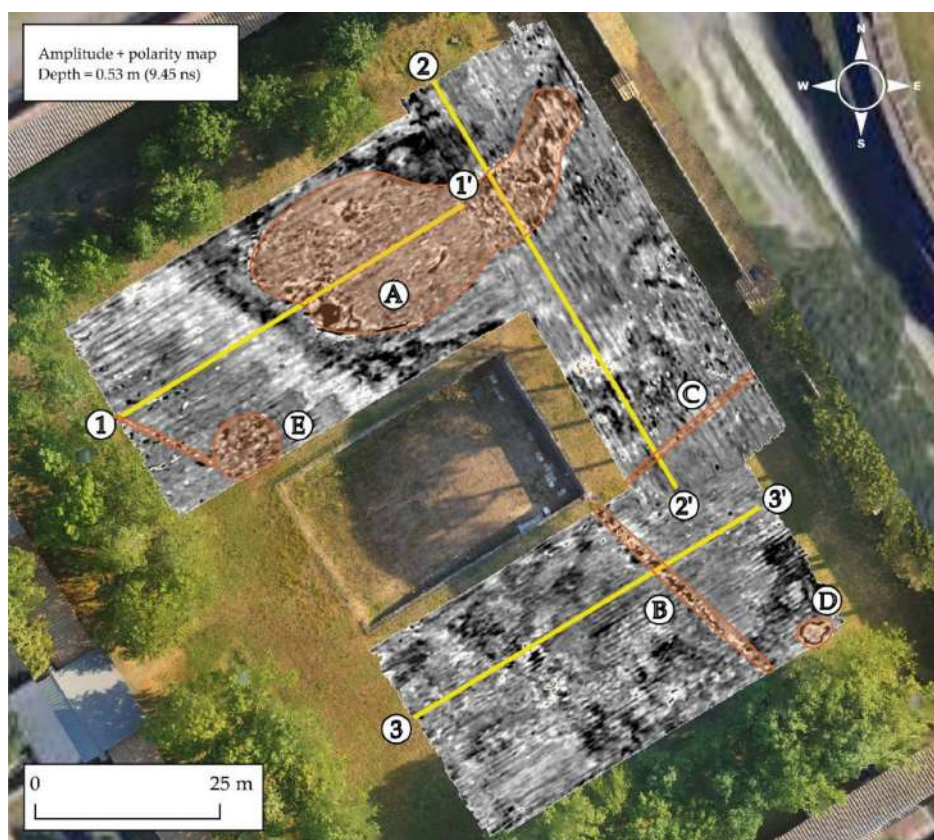
FIGURE 11 | Kirchhoff migration time-slice at 0.53 m b.g.l. (9.45 ns corrected return time). Notable anomalies are highlighted in orange, whereas B-scan sections 1–1', 2–2' and 3–3' are marked in yellow.
