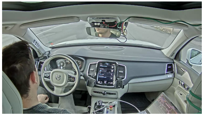
Figure 15. View of the test vehicle that is being controlled by solving Problem (4) on a laptop computer, and sending actuation requests over a network connection through OpenDLV.
