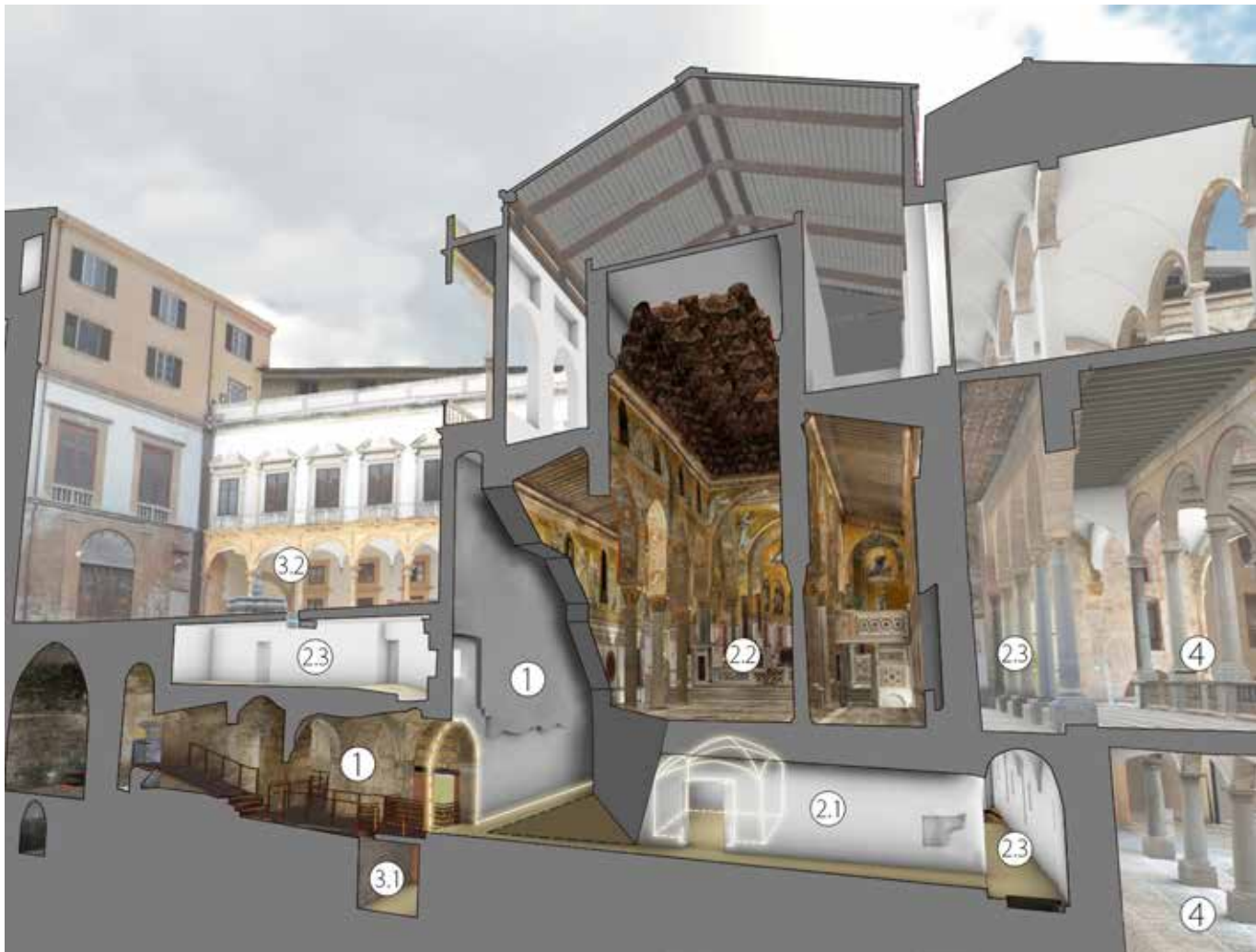
14 Axonometric cross section from the three-dimensional model of the Royal Palace (Graphic: TecnoArt) 1: pre-Norman phases (Segrete); 2: Cappella Palatina (1130); 2.1: lower church, with corridors and sacellum ; 2.2: upper church; 2.3: southern porticoes and northern buildings; 3: modern phases: 3.1: modern corridor (16th century, last quarter); 3.2: Cortile della Fontana (1571–1619); 4: Cortile Maqueda (1598–1610)
