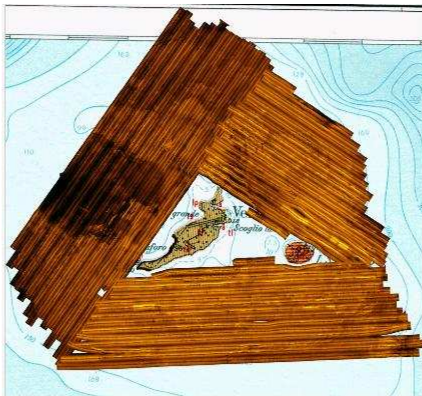
Figure 2 Mosaic of the sonar lines followed for survey around Ventotene and Santo Stefano. (Image courtesy Aurora Trust 2009).
