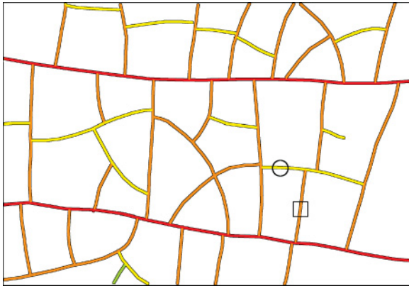
FIG. 9. (Color online) Edge ranks computed for the fracture pattern of Fig. 1. The root edges for rank computation are the two horizontal lines that cut the whole figure. The color coding is the same as for other figures. The \square and \circ symbols are referred to in the main text.
