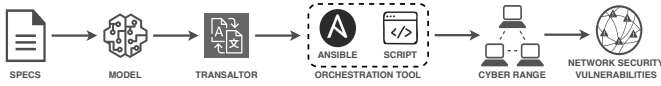
Figure 6. Graphical depiction of the working pipeline adopted to perform vulnerability assessments using a cyber range.
