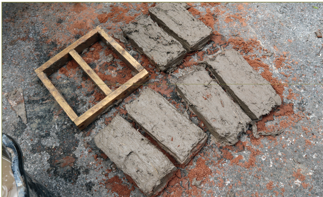
Fig 3. The adobe bricks made of clay tempered with dry straws. Photo by Tomei and Jiménez Rivero.
