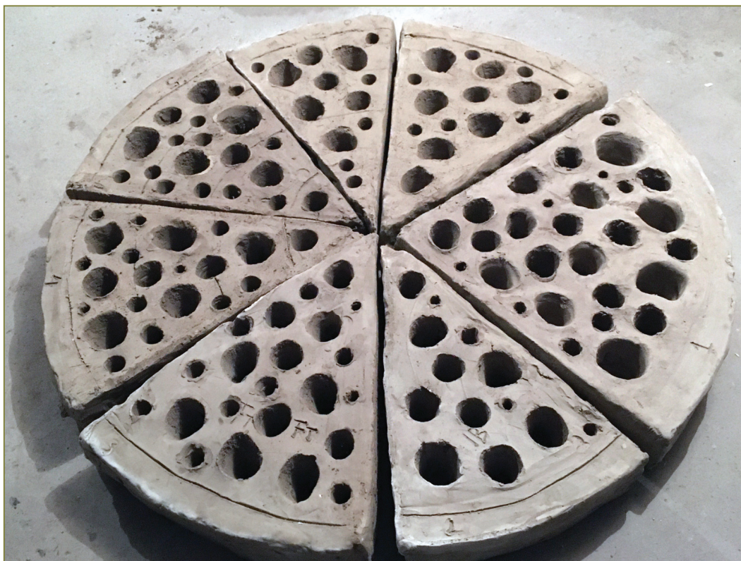
Fig 4. The perforated floor completed and dried out. Photo by Tomei and Jiménez Rivero.
