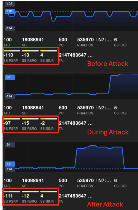
Figure 40: Measured power levels of reference signals (RSRP, RSRQ, and SINR) using the smartphone application before (top), during (middle), and after (bottom) the meaconing attack.
