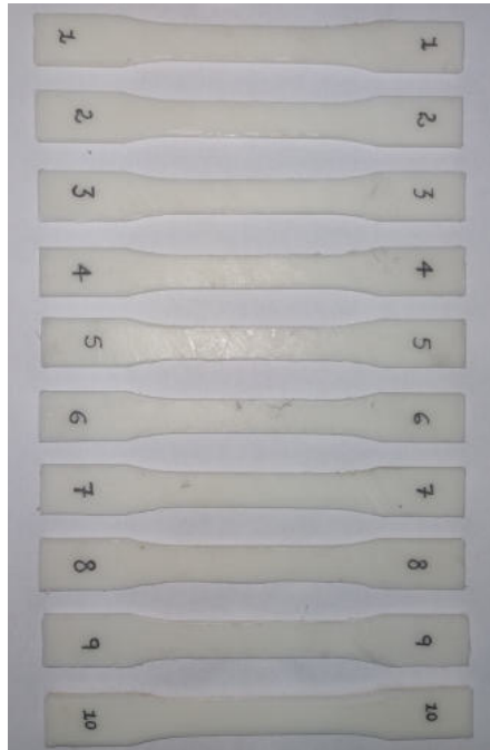
(a) Dog bone specimens for the tensile tests
