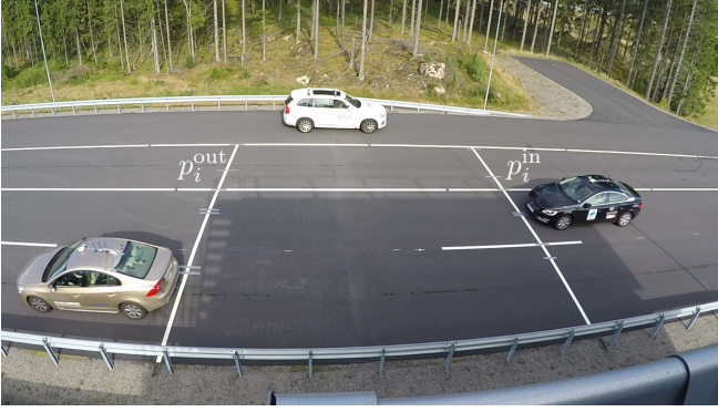
(a) Photo of the parallel configuration used in the experimental validation. The white lines mark the beginning and end of the intersection, p_i^{\text{in}} and p_i^{\text{out}} , and collisions are thereby avoided when only one vehicle is between the two white lines at a given time.
