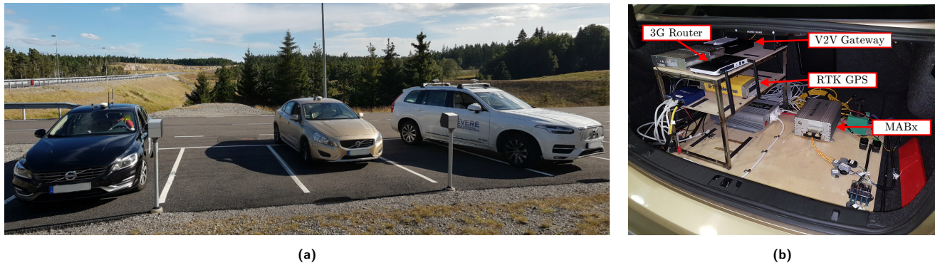
FIGURE 3 Photos of the experimental hardware platform. (a) Shows the three vehicles used, (b) Shows the hardware installation in one of the vehicles. The 3G router was used to provide an IP link for the RTK corrections used by the GPS receiver
